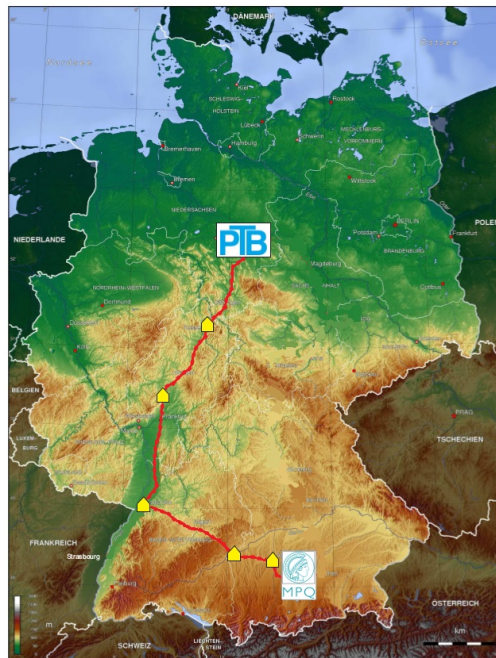
Figure 1: Simplified scheme of optical fiber connecting MPQ and PTB institutes. Yellow markers stand for the amplifiers.
