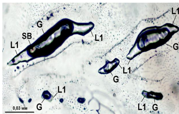
Figure 4. Change of relation of phases in the large inclusions and appearance of numerous secondary inclusions around them.
