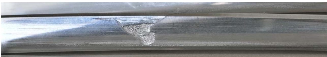
Fig.13. Trochoidal interference due to lead crowning and flaking failure
