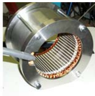
Fig.7, DC motor stator
