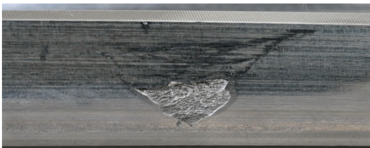
Fig.2. Middle stage of flaking progress
