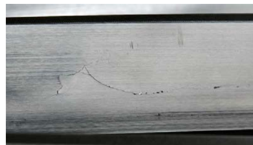
Fig.3. Crack on back flank of the tooth
