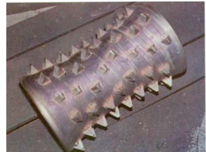
Figure 9. Toroidal hob to envelop the TP worm gear.
