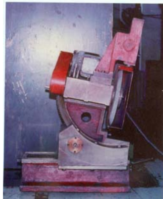
Figure 8. Grind unit to generate the TP worm.
