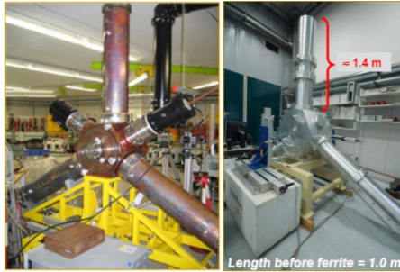
Figure 4: Accelerating cavity of the BESSY accelerator (left) and ESRF (right).
