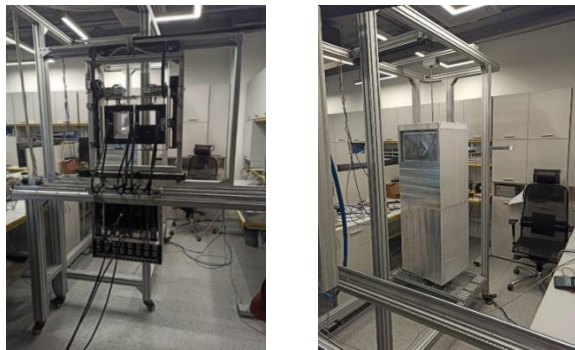
Figure 5: The positioning system of the ISCRA station (left) and energy degrader (right).
