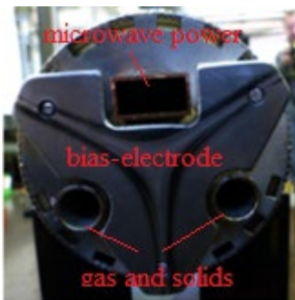
Figure 2: Injection plug of the DECRIS-2M ion source with new inputs: microwave power, gas and solids.
