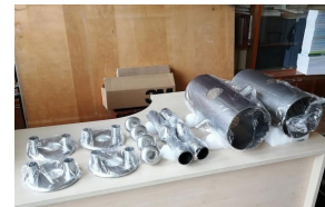
Figure 10: Nb parts for two Nuclotron-NICA cavities.
