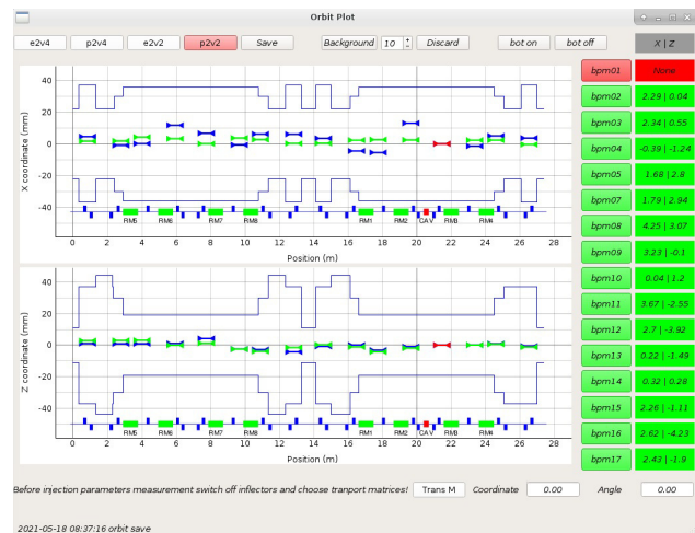
Figure 4: Displaying damping ring beam position. Green marker is the last measured beam coordinate, blue marker is the saved position, red is the inactive BPM's.
