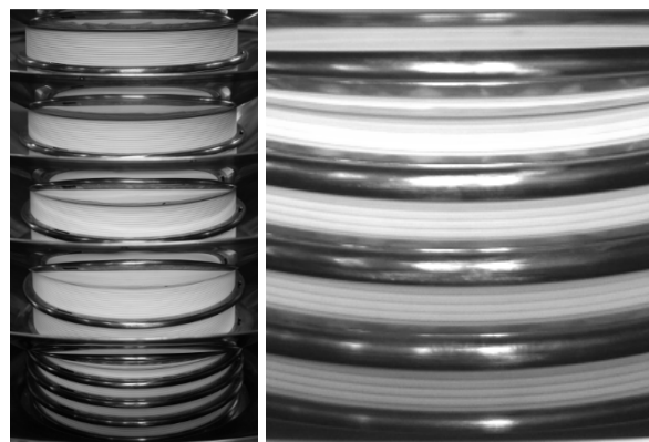
Figure 7: Ribbed ceramic surface (left, right) after training without breakdown traces.
