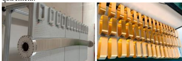
Figure 10: ceramic-lined thin-wall vacuum chamber for BRing dipole (left) and the ceramic rings inside.
