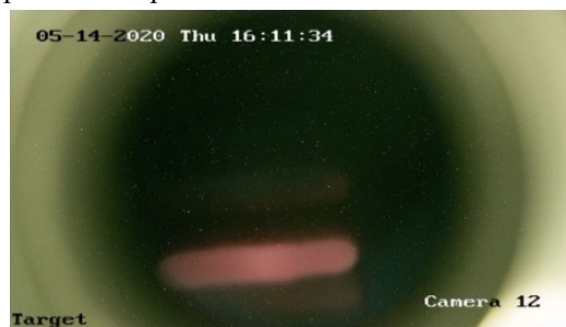
Figure 4: The argon beam glow and a beam of neutral atoms caused by the luminescence of the target lithium layer upon a twofold increase in the argon flow in the stripping target.
