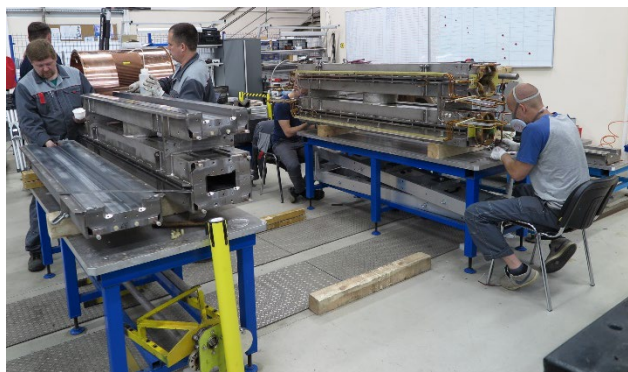
Figure 5: Preparation the magnet to cryogenic test.
