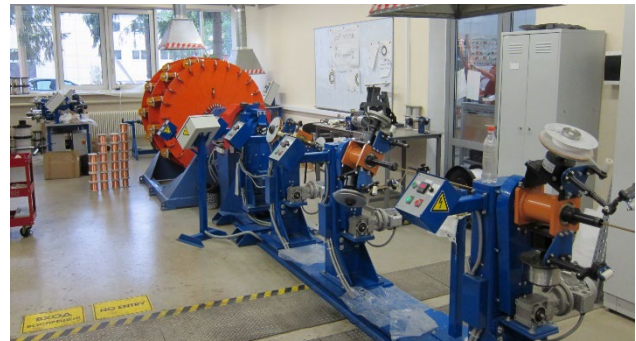
Figure 2: Cabling machine for the manufacture of a hollow composite SC cable.
