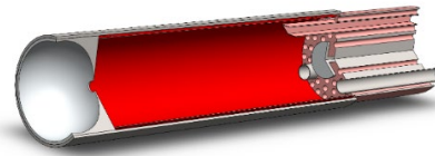
Figure 6: DECRIS-PM vacuum chamber, a hot tantalum screen is red.
