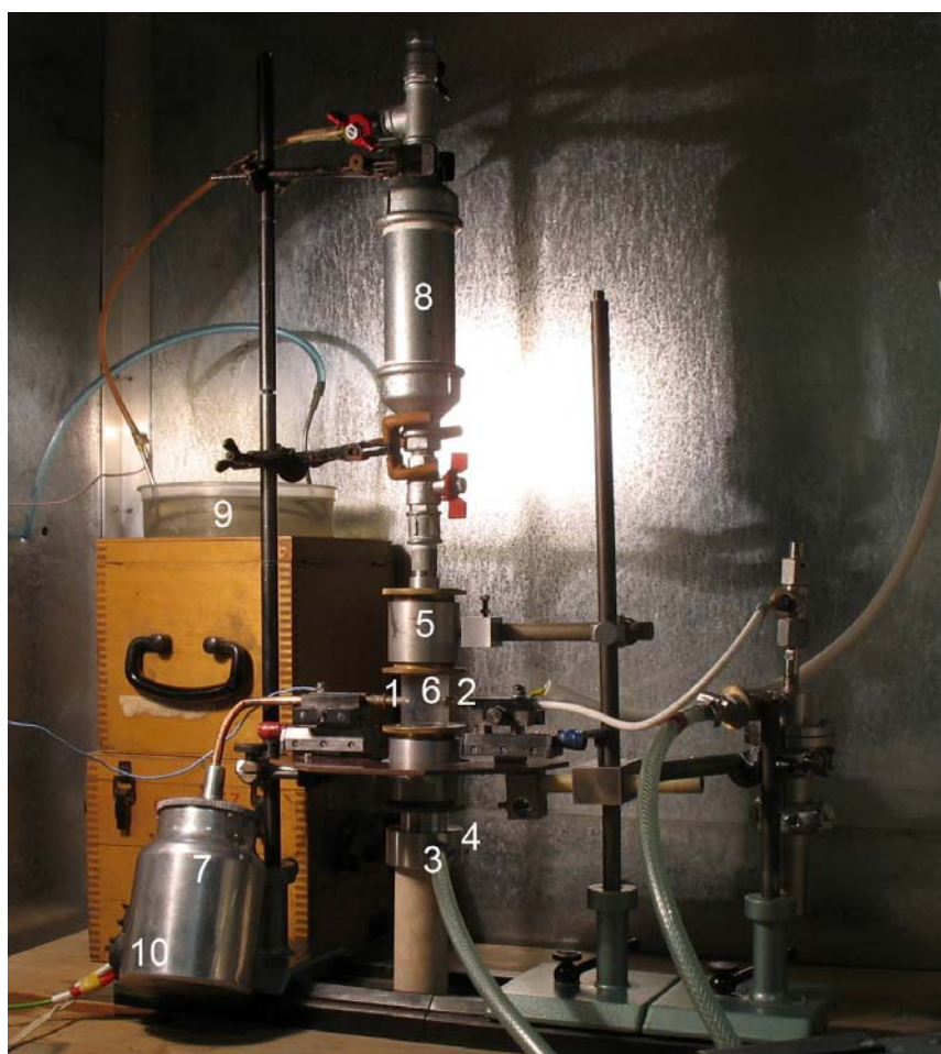
Figure 2. General view of the experimental set up. 1,2- tube electrodes - injectors for H_2O+Al , 3,4- nozzles – injectors for argon flow, 5-reactor chamber; 6- quartz tube; 7-water steam generator; 8- gas silence chamber; 9- water cooling tube; 10- electric heater
