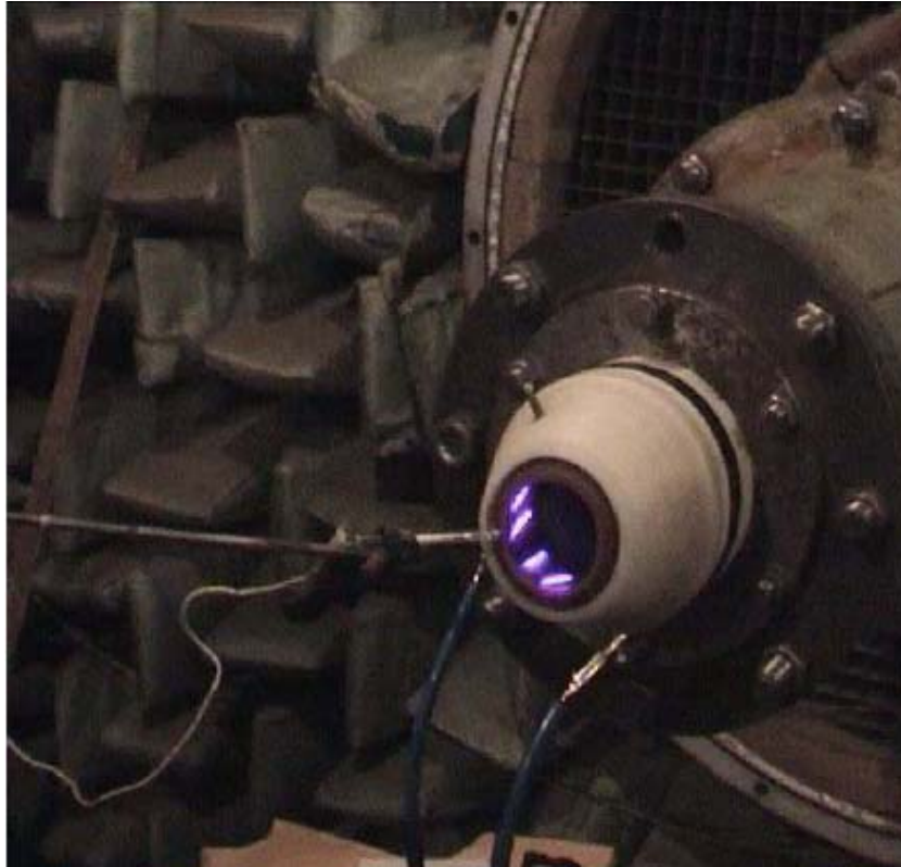
Fig.2. Subsonic nozzle with operating CHFD actuator ( P_{st}=1 Bar, V_j\sim 100 m/s)
