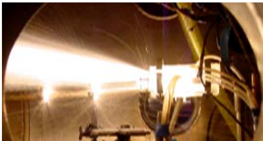
Figure 6. The general view of the combined discharge created in a high speed propane-air stream in a rectangular cavity with angled rear-wall on a wide wall of the aerodynamic channel.
