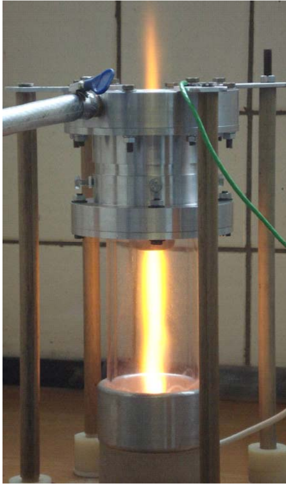
Figure 3. Plasma chemical reactor with pulsed repetitive HF discharge in H 2 O-Al mixture
