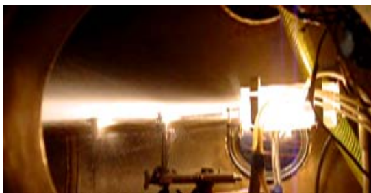
Figure 7. The general view of the combined discharge created in a high stream of propane-air ( M=2 ) in a rectangular cavity with various depths of forward and back walls on a wide wall of the aerodynamic channel at microwave pulse duration \tau=10^{-5} s, repetition frequency f=100 Hz, duration of direct current discharge t=1 s, and time exposure is 20 ms. The propane-air flow is directed from right to left.
