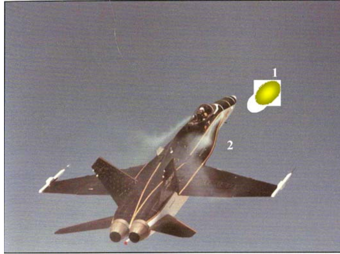
Figure 5. Possible control of conical vortex parameters near plane by plasma formation at large attack angle. 1- HF plasmoid, 2-conical vortex
