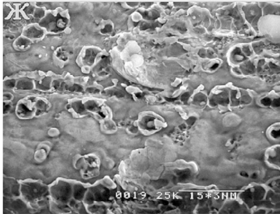
Fig.16. Surface morphology integrated over experimental activity with deuterium-loaded Pd anode (fragment 1, “coronal” anode; particular part of Pd tube, which is close to Cu head-end of anode, scale 60 μm).
