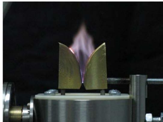
Fig. 1. Principle of gliding arc operation and integral photograph of discharge luminosity ( R_b=10 \text{ kOhm} , C_c=300 \text{ pF} , V_0=3 \text{ kV} , R_{sh}=1 \text{ Ohm} ).
