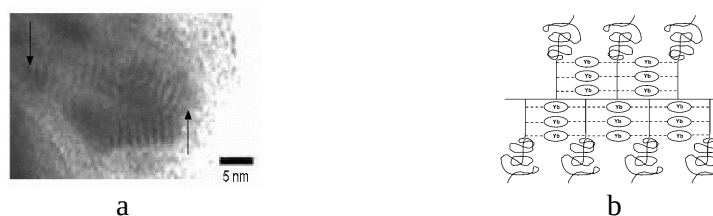
Fig. 1. (a) TEM micrograph and (b) schematic representation of the architecture of a conjugate between PI-g-PMAA molecular brush and Yb(III)-porphyrizine complexe.
