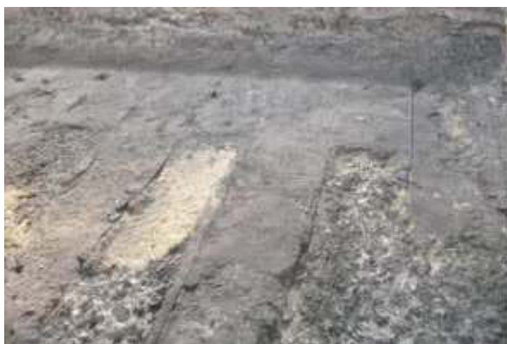
Fig. 3 Delaminated cathode carbon blocks caused by substitution of low quality raw materials [2]
