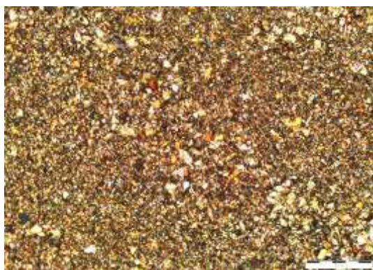
Fig. 3. Gold particles appearance, shape and size of cyclone underflow flash-flotation concentrate at «Verninskaya» plant. Minimal size units are \mu\text{m} , maximum size – 300 \times 500 \mu\text{m} .
