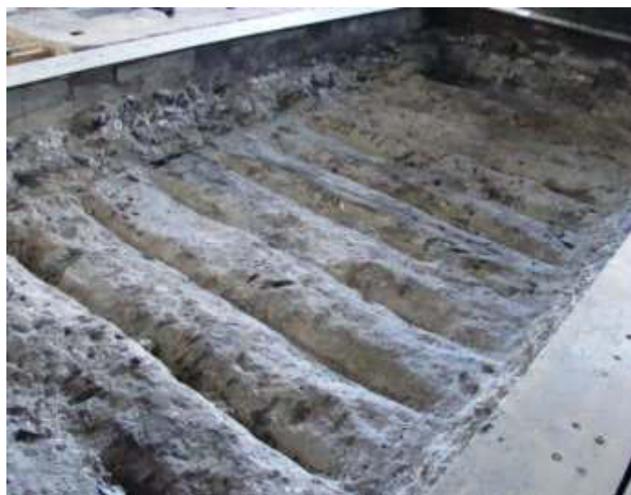
Fig. 1. Electrolysis pot with recovered cathode
