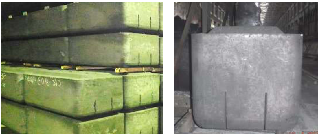
Fig. 12 “New” optimized anode with chamfered edges
