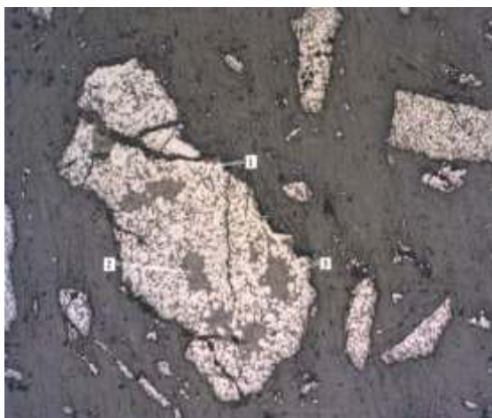
Fig. 4. General view (x50 magnification) of the uptake build-up sample: 1 – trevorite; 2 – Ca and Fe aluminosilicate; 3 – silicate
