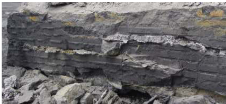
Fig. 5. Metal infiltrations in the horizontal cracks of a domestic cathode.
