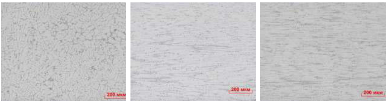
Fig. 5. Microstructure of cast item, pressed rod, wire rod, alloy 4043.
