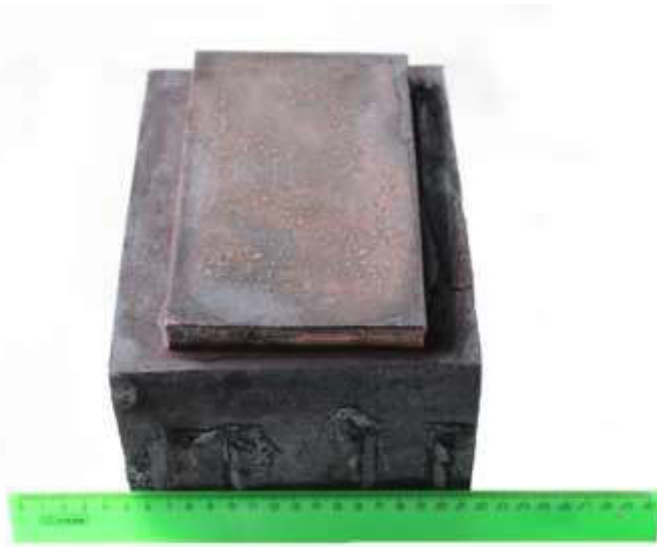
Fig. Bimetallic steel-copper sample obtained by mode 3
