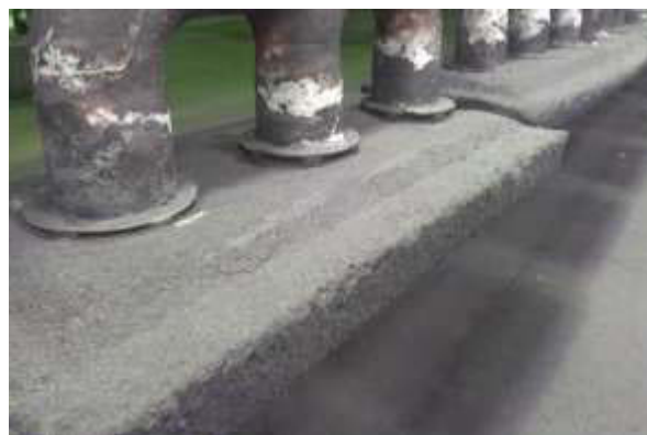
Fig. 8. Anode butt with 50 mm “lip”
