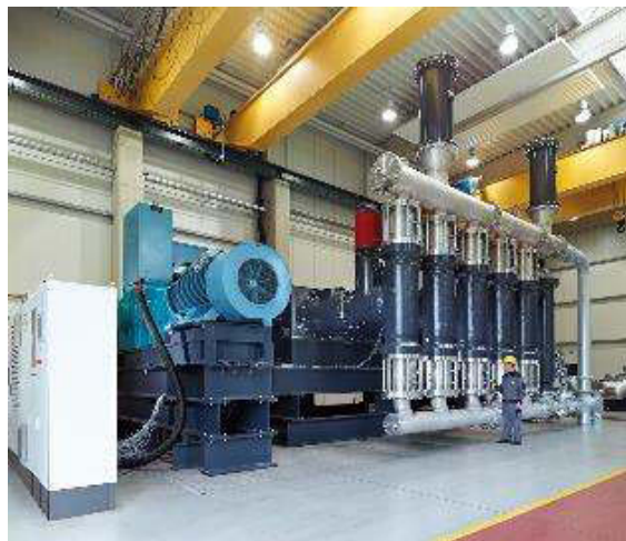
Fig. 11. MULTISAFE double hose-diaphragm pump in quintuplex design with a maximum flow rate 1,000 m 3 /h
