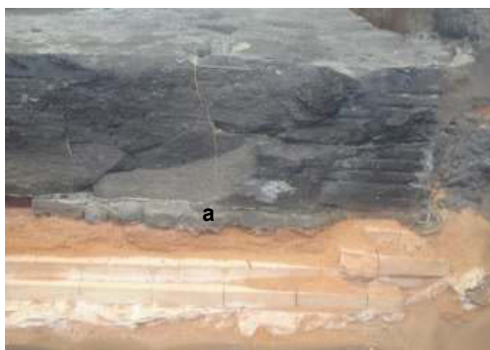
Fig. 6. DIM with properly formed barrier (a) and unreacted material below
