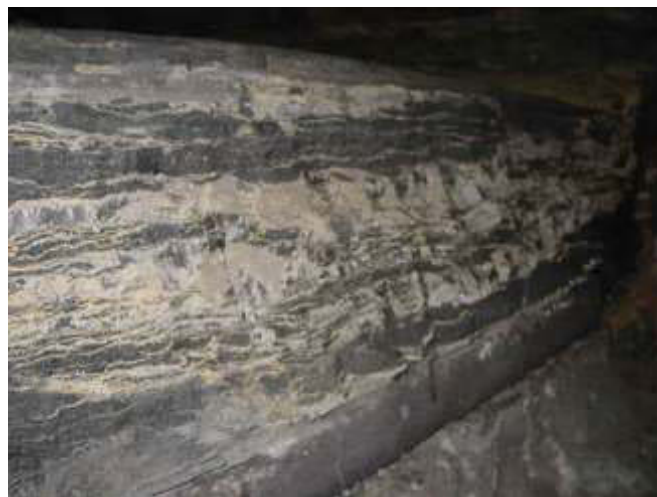
Fig. 2. Cathode block with severe horizontal cracking and penetration of metal. Failed at about 180 days
