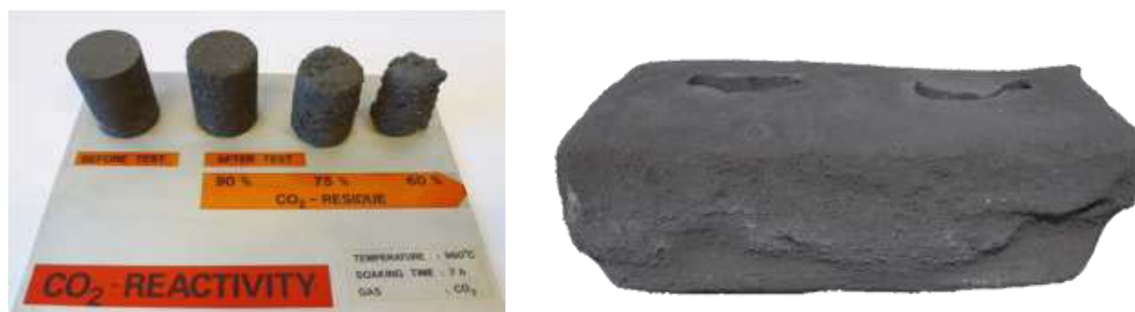
Fig.3. Test specimen before and after the CO 2 reactivity test; anode with severe CO 2 attack
