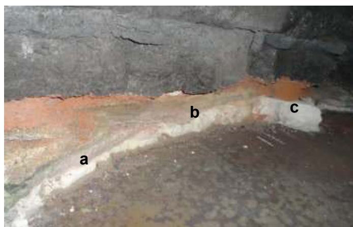
Fig.7. Refractory and insulation beneath block at center of pot: a) Penetrated DIM; b) Penetrated CaSi; c) CaSi still 8 cm at center
