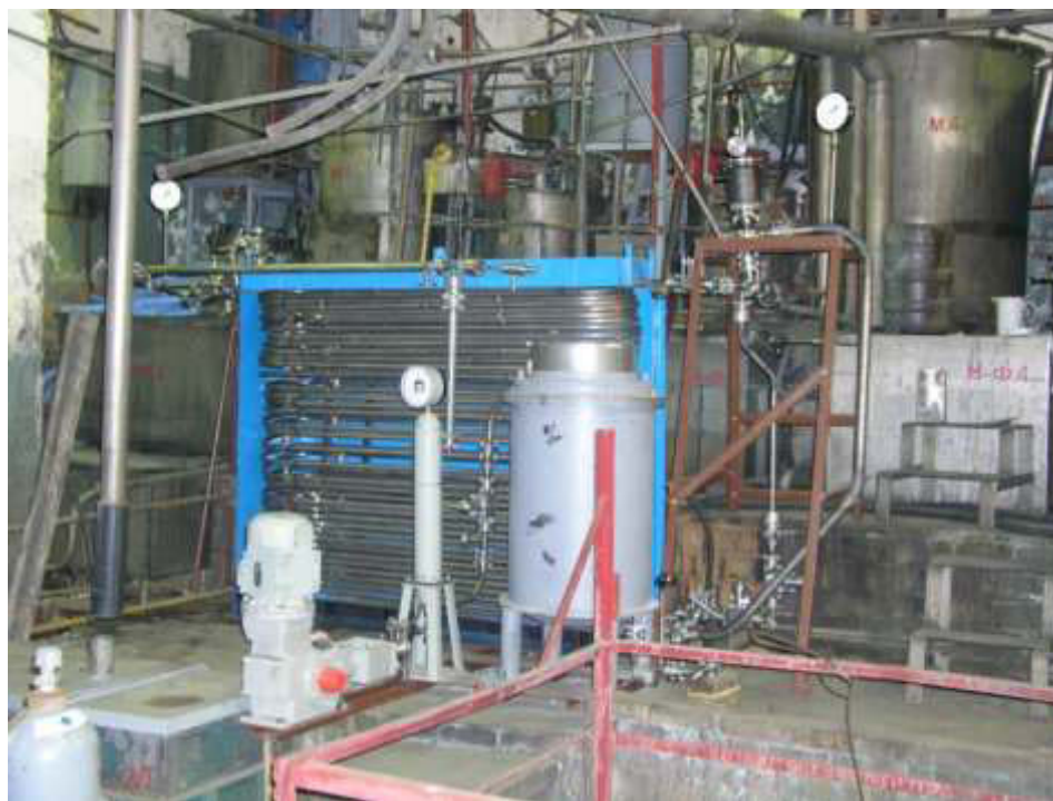
Fig. 3. High-temperature leaching unit (developed by Kaminsky Yu.D. (Ph. D. (Chemistry)) et al. [11])
