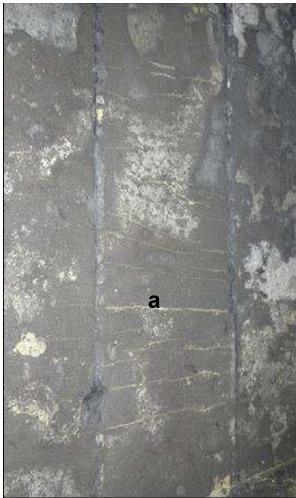
Fig. 5. Excessive cracking (a) of cathode blocks, leading to development of potholes (b)
