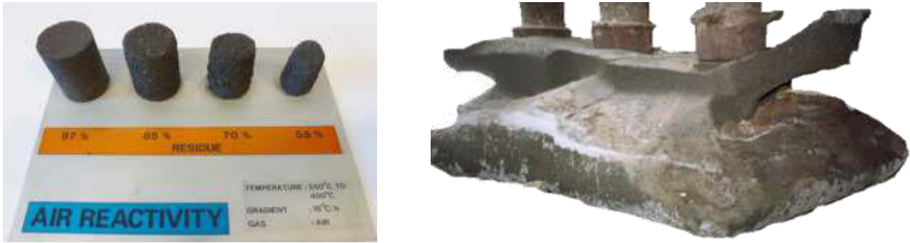
Fig. 4. Test specimen before and after the air reactivity test; anode with severe air burn attack
