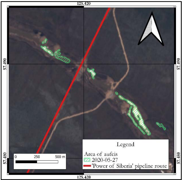
Fig. 2. Ice massifs on the Tit River near the route of the ‘Power of Siberia’ pipeline (May 27, 2020)
