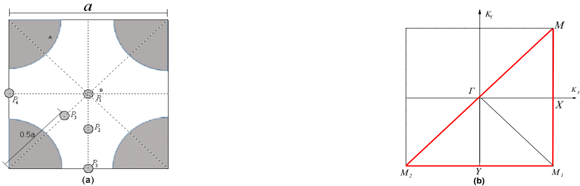
Fig. 1. (a) Unit cell for MCs of the square lattice with two rod in it, (b) The first BZ for the square lattice shown in Fig. 1(a), where red lines indicate the four triangles studied.
